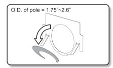
2. Release two clips on both sides of the luminaire to open the cover.
