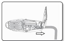
**5.** Rotate the luminaire to the desire position and angle.
