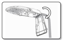
**6.** Screw the bolts of the luminaire tightly.
